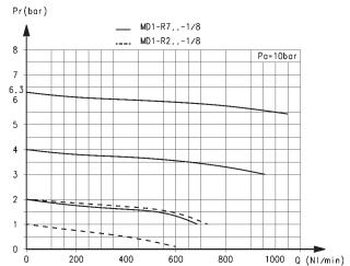
Ports with interchangeable 1/8 threaded cartridges
